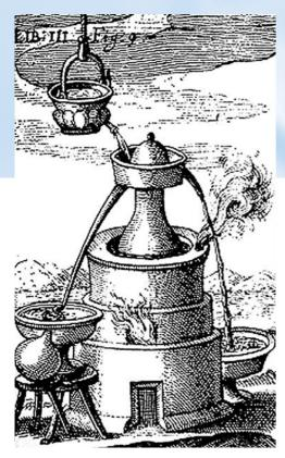
Alambic with water cooling around the distillation helmet.
